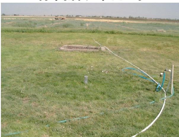
Figure 3- Grass lysimeter with FDR access tube
