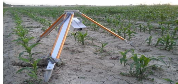
Figure 1- The scanner used for insolation simulation of maize plants
